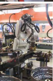
This machine permits the assembly and the relative test of all the standard valves up to 1". For each assembled valve an automatic report that shows every step of the process is made, thanks to the pictures shot by the cameras placed in each station of the machine.
